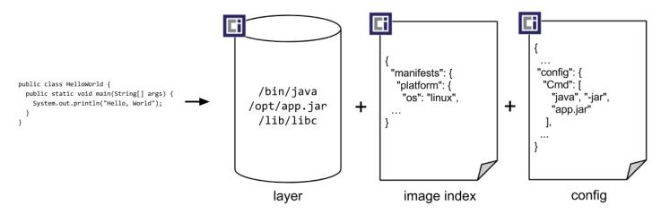
Once built the OCI Image can then be discovered by name, downloaded, verified by hash, trusted through a signature, and unpacked into an OCI Runtime Bundle.
